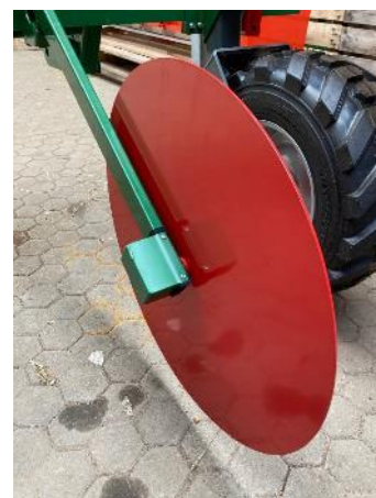
Protective disc with speed sensor
