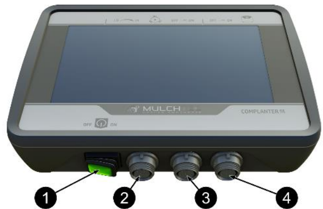
The connections of the control panel
