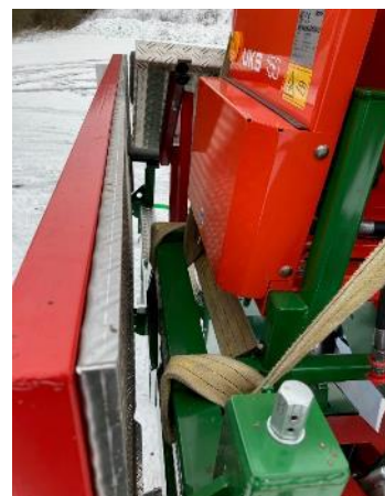
Lifting with slings around the side frame
